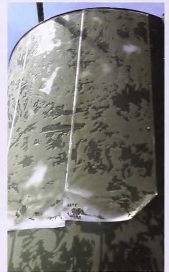
Affix the stencil, and apply the second color.
